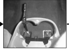
**STEP 15:** Using an an 18mm socket wrench, secure the front of the console to the vehicle with the 18mm bolts removed in Step 1.
